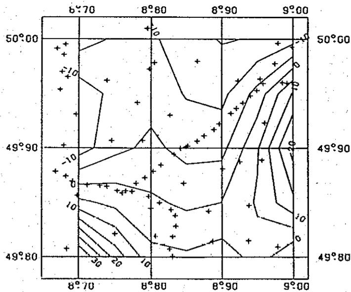
Fig. 1b. The position of the stations and the surface values of density anomalies (the absolute density -  $2.67 \text{ gcm}^{-3}$ ). The units of density are  $0.01 \text{ gcm}^{-3}$ .
