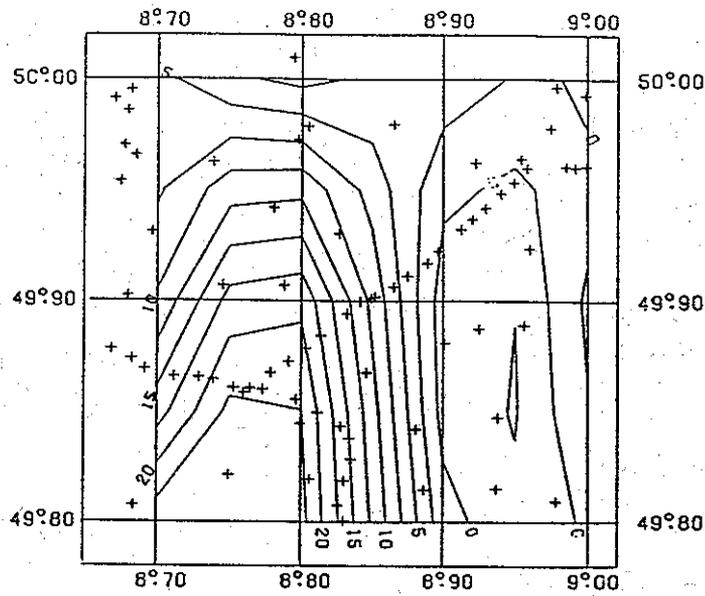
Fig. 1a. The position of the stations in the area and the bouguer anomalies (in mgal).
