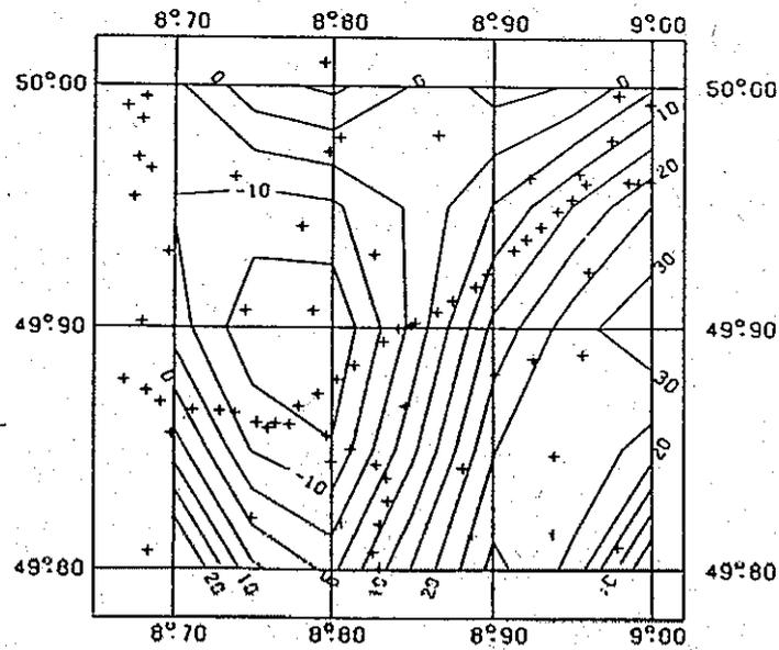
Fig.5. The differences between the predicted- and the measured density anomalies in units of  $0.01 \text{ gcm}^{-3}$ . The parameters of the model are : ( $R-R_B = 5500 \text{ m}$ ,  $m = 1100$ ,  $C_{\Delta g \Delta g}(0) = 104.00 \text{ mgal}^2$ ).
