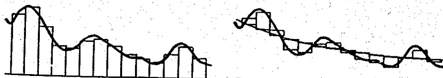
Fig. 2. Modeling the topography (left) and the residual topography (right) with rectangular prisms. In the RTM reduction, masses above the mean elevation surface are removed, while valleys are filled (prism density negative).
