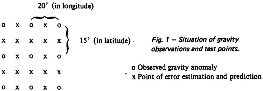
This kind of prediction situation may be most efficiently handled using stepwise collocation, cf. Moritz (1973) and Tscherning (1974a). The datasets  $x_1$  and  $x_2$  are used to determine two harmonic functions  $\tilde{T}_1$  and  $\tilde{T}_2$ .
