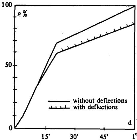
*Fig. 7 – Variation of the ratio,  $\rho$ , for the mean gravity anomaly of the square for varying spacing  $d$  of the fictitious observed  $\Delta g$  with and without a pair of deflections in each corner. The covariance function (17b) was used.*
