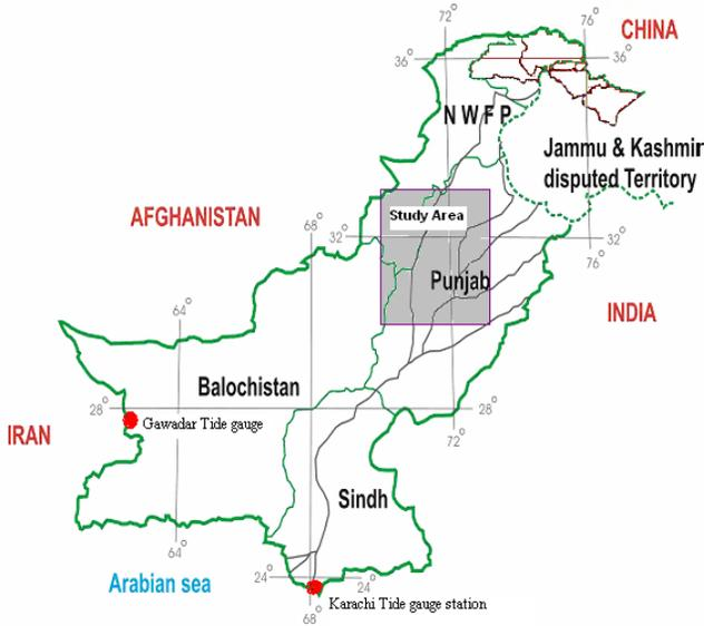
**Fig. 2.** Study area bounded by the rectangle. Two tide gauge stations at Karachi and Gawadar are main tide stations used for GPS-Levelling network with Karachi being the reference Tide station.
