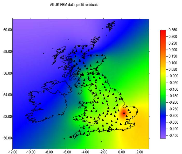
Figure 7. Differences in metres between the 180 point values of the Newlyn-ellipsoid separation and the geoid
