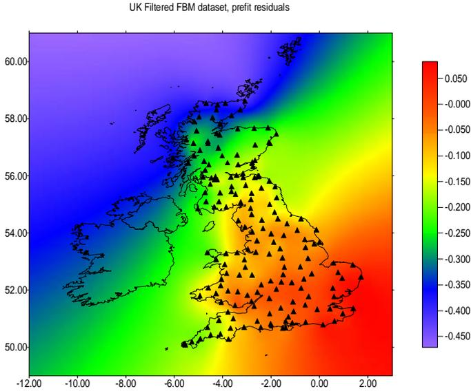
**Figure 8. Differences in metres between the remaining 179 point values of the Newlyn-ellipsoid separation and the geoid**
