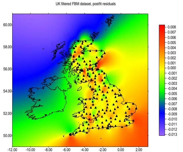
**Figure 9. Post-fit residuals after modelling of the difference between the GPS-levelling and the de-trended geoid**
