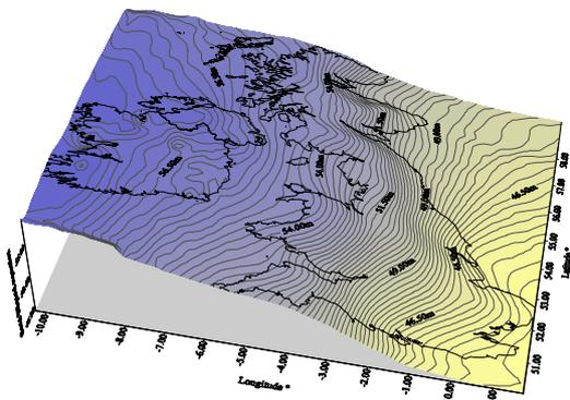
Figure 6. OSGM02 geoid with respect to the GRS80 ellipsoid
