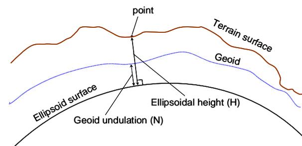
**Figure 1: The relationships between the geoid, an ellipsoid and the terrain surface.**
