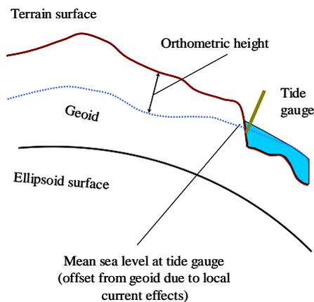
**Figure 2: Mean sea level and the geoid are not necessarily coincident at any one particular tide gauge.**
