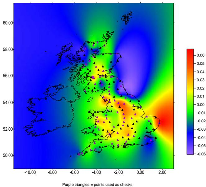
**Figure 10. Corrector surface fitted to subset of 100 data points (black triangles) and checked against remaining network stations (purple triangles)**
