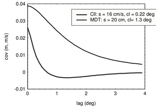
Figure 4. Covariance functions of the MDT and the geostrophic surface current components based of the MDT degree variance model shown in Figure 3.
