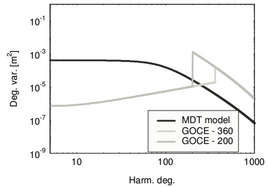
Figure 3. MDT signal degree variance model shown together with the geoid error degree variances associated with GOCE Level 2 harmonic expansion to degree 200 and to degree 360 simulating the collocation solution
