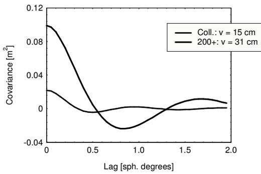
Figure 2. Geoid error covariance functions associated with GOCE Level 2 harmonic expansion to degree 200 and to degree 360 simulating the collocation solution
