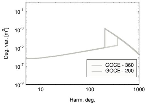
Figure 1. Geoid error degree variances associated with GOCE Level 2 harmonic expansion to degree 200 and to degree 360 simulating the collocation solution
