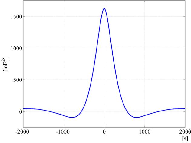
Fig. 4. Covariance function of the  $T_{rr}$  estimation error, using a single-input single-output Wiener filter.
