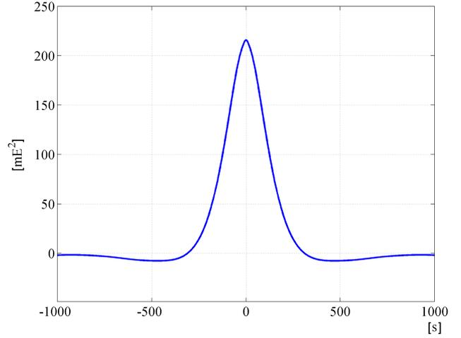
Fig. 5. Covariance function of the  $T_{rr}$  estimation error, using a joint Wiener filter between  $T_{rr}$  and  $T$ .
