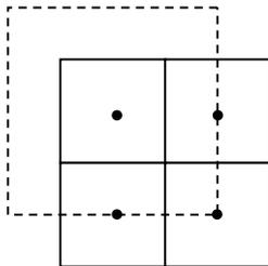
Fig.2. Interpolation scheme: in solid line the final grid and in dashed line the moving window used for estimating the centre value of each cell.
