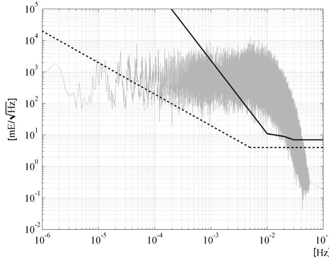
Fig. 1. Signal (in grey) and noise (in black) power spectral density of the  $T_{zz}$  component. Original performance (in dashed line) vs. new specification (in solid line).
