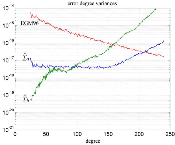
Fig. 6. Estimation error of the harmonic coefficients using numerical integration with  $T_{rr}$  gridded data ( $\hat{T}_a$ ) and with  $T$  gridded data ( $\hat{T}_b$ ). The reference model is EGM96.
