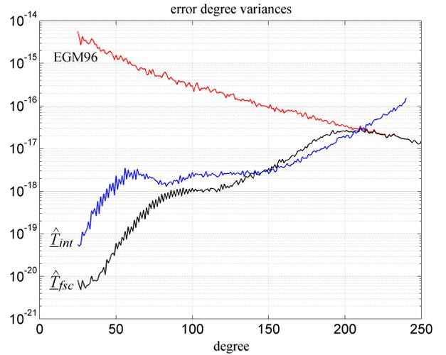
Fig. 7. Final estimation error of the harmonic coefficients using fast spherical collocation ( $\hat{T}_{fsc}$ ) and numerical integration ( $\hat{T}_{int}$ ). The reference model is EGM96.
