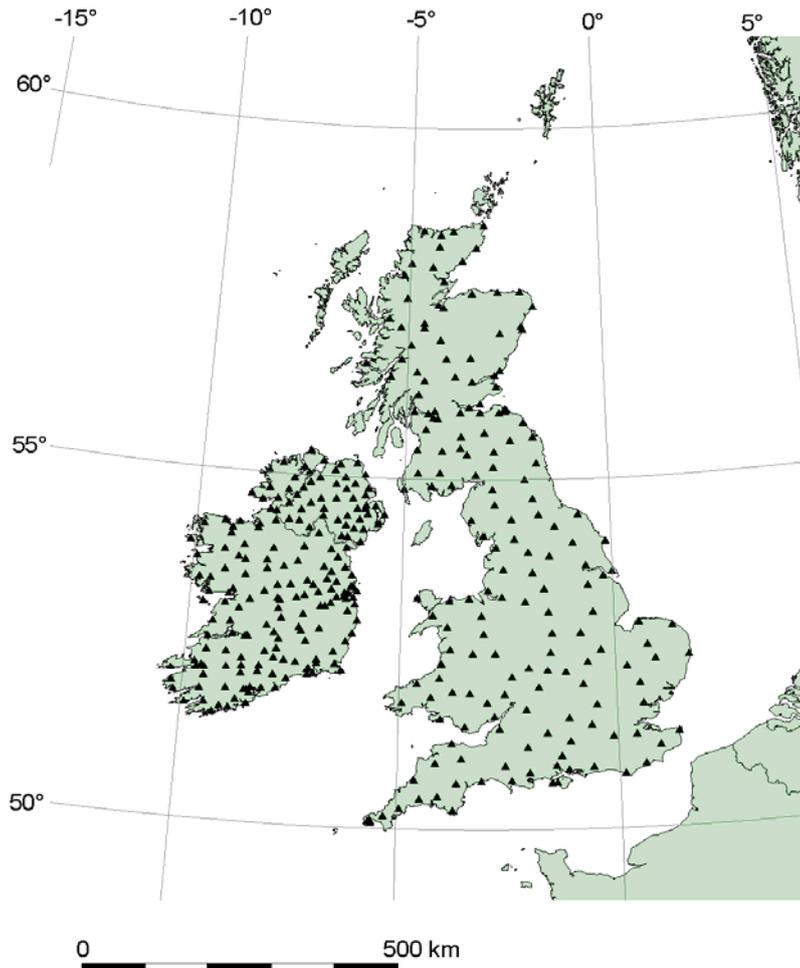
Fig. 3. GPS and levelling points available for fitting.
