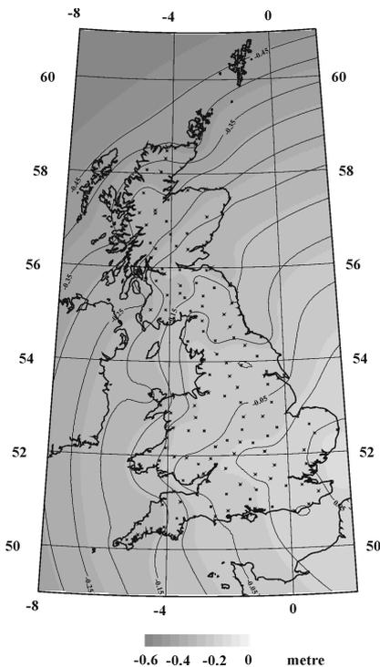
**Fig. 6.** Location of 179 ODN GPS/levelling points used in post-fit GPS/levelling statistics and the modeled geoid fit surface  $\epsilon$ . Contour interval: 0.05 m.
