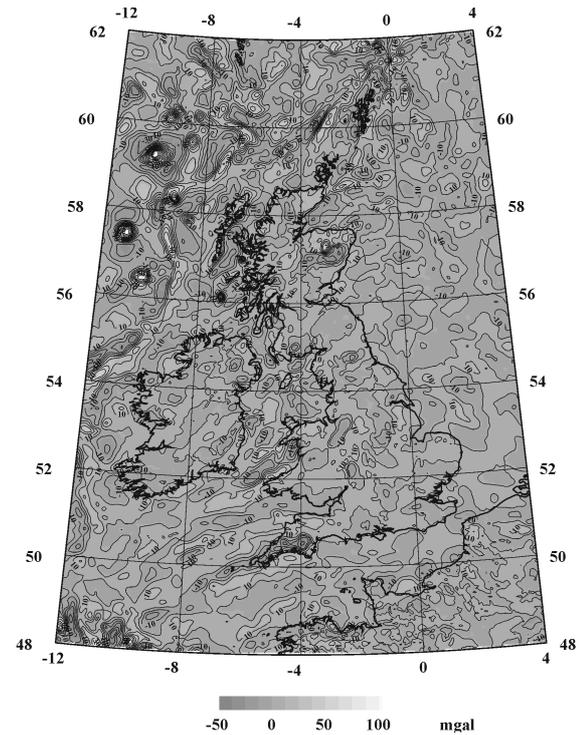
**Fig. 4.** Residual free-air gravity anomalies  $\Delta g_{\text{res}}$ .
