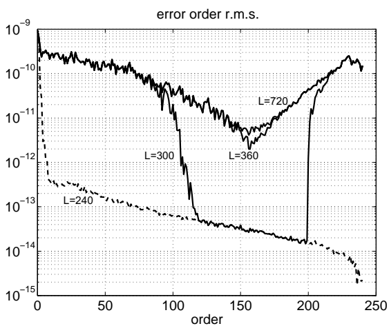
Fig. 11. Numerical integration error order r.m.s. as a function of the maximum degree L . For values of L close to the Nyquist limit, the aliasing only spreads at low and high orders; increasing the values of L , it quickly becomes stable. The dotted curve represents the error order r.m.s. without aliasing
