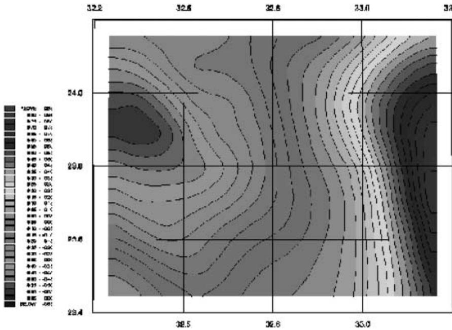
Fig. 6. Residual LSC geoid from gravity and GPS/levelling c.i. 0.05 m
