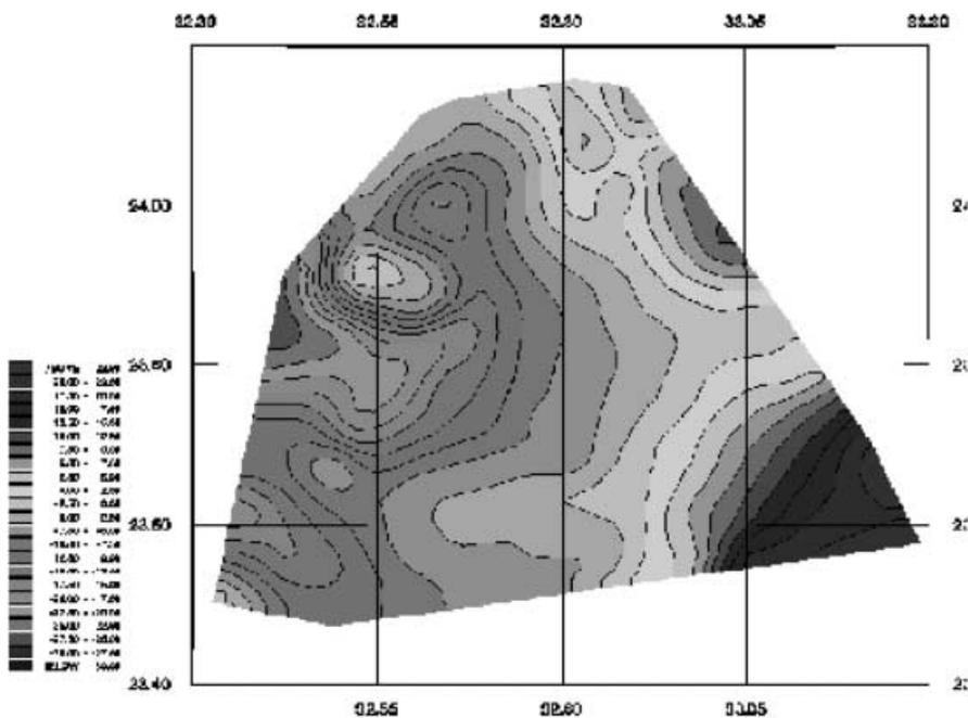
Fig. 4. Gravity disturbances EGM96. Contour interval 2.5 mGal
