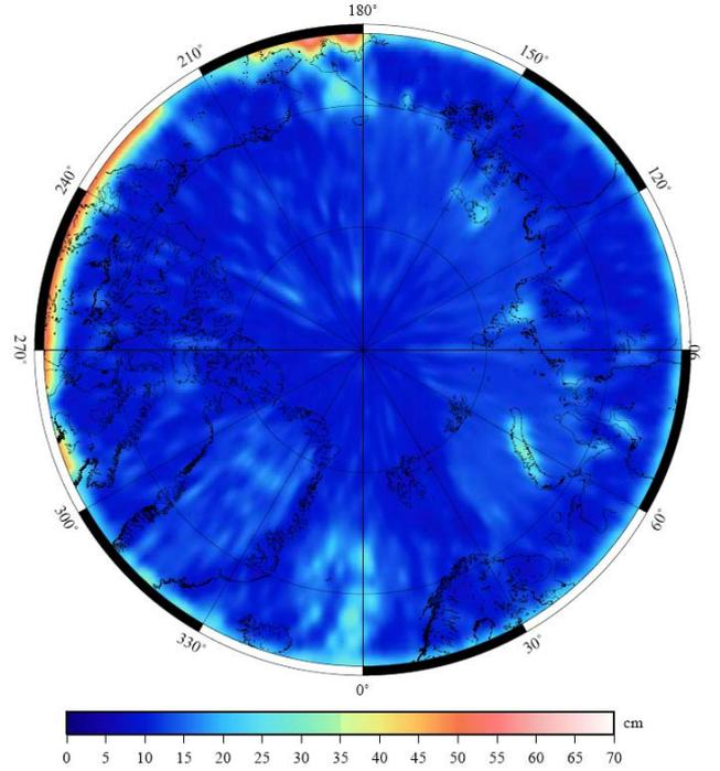
Fig. 4. Geoid error estimates from collocation. Unit cm.
