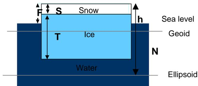
Fig 1. Sea-ice freeboard  $F$ , thickness  $T$  and its relation to geoid  $N$ , MDT (sea level minus geoid) and mean sea level.
