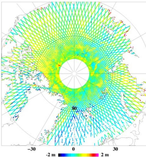
Fig. 6. Difference ICESat SSH (laser 1) minus the geoid.
